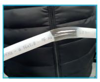
SharkBite PEXa tubing due to its excellent thermal memory absorbs the increase in size due to freezing. Crosslinking by the PEXa system (peroxide method), allows it to expand (due to the increase in volume due to freezing) and absorb much of the expansion energy of the freezing process. No pipe is completely immune to freezing, but RWC's SharkBite PEXa pipe is extremely resistant to freezing damage.
